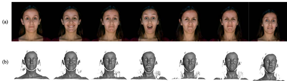
Fig. 3 Example of acquired data using the 3D scanner: (a) frontal faces with different expressions of one subject, (b) corresponding face geometry
