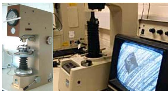
Fig. 1. Hardness testing machines.
